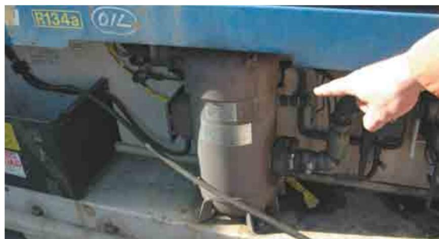
**Potentially dangerous:** Container companies saved money by using cut-rate contractors in Vietnam to service refrigerator compressors like this one. The decision led to the deaths of three dockworkers and triggered an expensive global safety problem when compressors began exploding.
